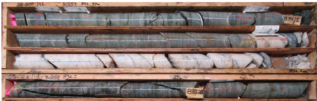
First hole of the program SB-2018-014A: Intersected 29.56 g/t Au over 0.88 m true width containing visible gold
