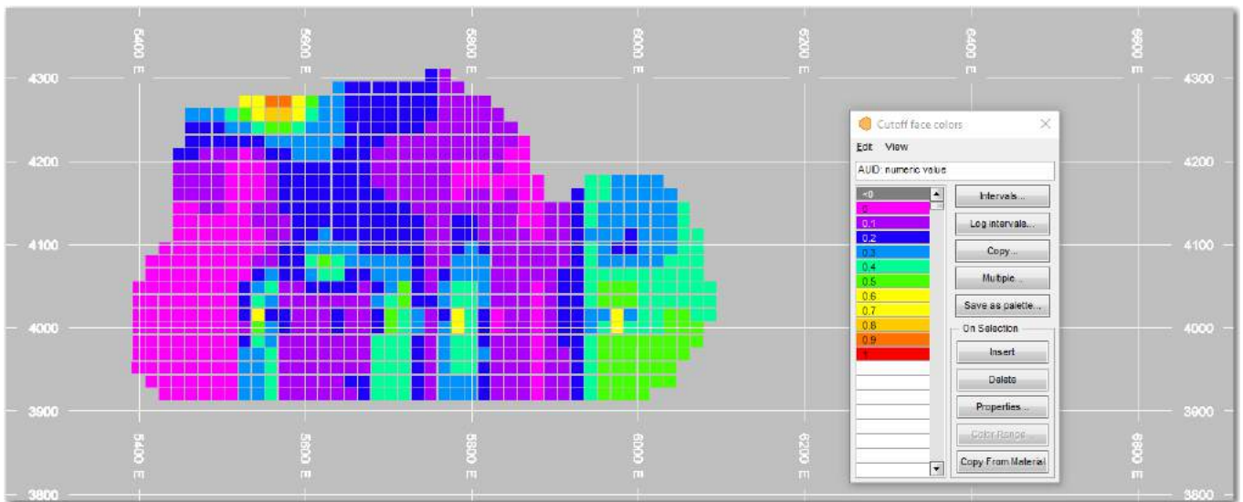
Figure 14-10: Long-section View of Shaft Vein Block Model looking North (grid lines=200')
