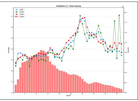
Figure 14-29: Avino Vein, Swath Plot for Copper, Elevation (Red Pennant 2022)
