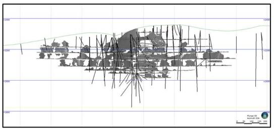
Figure 6-2: San Gonzalo Mine: Vertical Section View Showing Development and Stoping (Red Pennant 2022)
