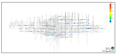
Figure 9-2: Channel Samples, Colour Coded by Silver Grade, within the San Gonzalo Vein System
