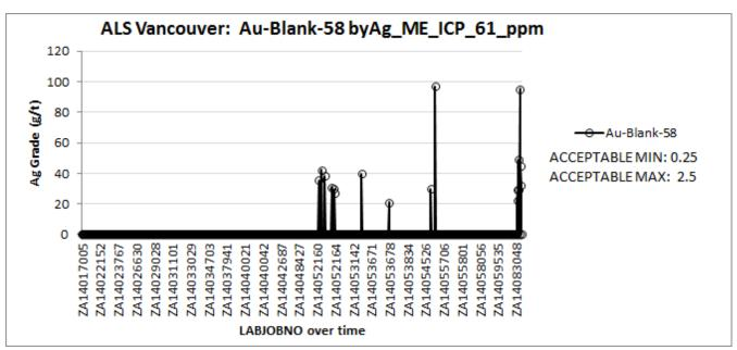
Figure 11-25: Silver Blanks. Large Population with Multiple Failures of Large Magnitude. Baseline, or ACCEPTABLEMIN is 1/2 the LOWERDETECTION of the Assay Method.
