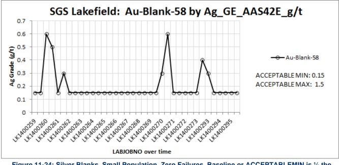
Figure 11-24: Silver Blanks. Small Population, Zero Failures. Baseline or ACCEPTABLEMIN is ½ the LOWERDETECTION of the Assay Method.
