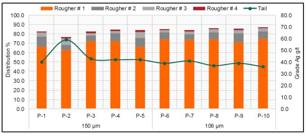
Figure 13-4: Silver Recovery – Bulk Rougher Flotation - Martha Composite (after SGS, 2021)
