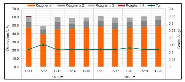
Figure 13-5: Gold Recovery – Bulk Rougher Flotation - Abundancia-Gloria Composite (after SGS, 2021)
