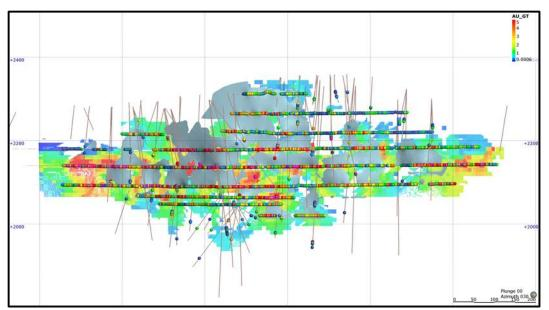
Figure 14-23: San Gonzalo Vein: Longitudinal Section Showing the Block Model Centroids Color Coded by Gold Grade (Red Pennant 2020)
