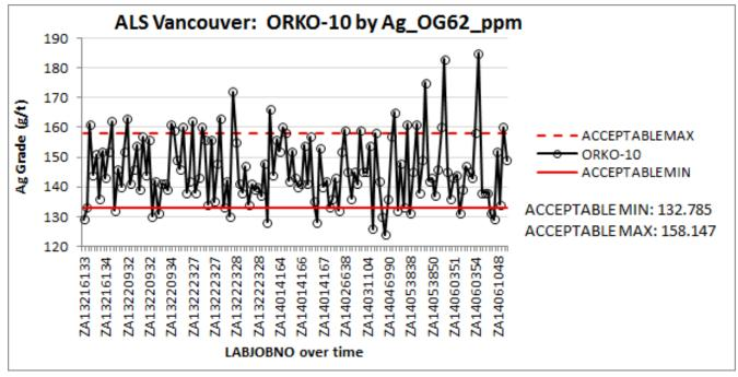
Figure 11-23: Orko-10 Silver Standard. Medium Population, with Multiple Failures Outside the Acceptable Minimum and Maximum.
