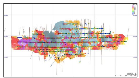
Figure 14-22: San Gonzalo Vein: Longitudinal Section Showing the Block Model Centroids Colour Coded by Silver Grade (Red Pennant 2020)
