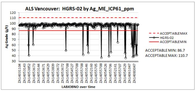
Figure 11-27: Silver Standard. Large Population with Multiple Failures of Large Magnitude Below the ACCEPTABLEMIN.
