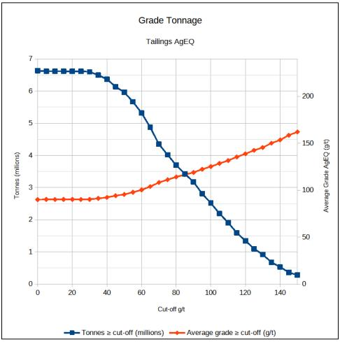
Figure 14-46: Tailings Material Grade Tonnage Graph
