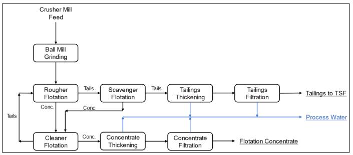
Figure 17-1: Simplified Flowsheet – Avino Processing plant
